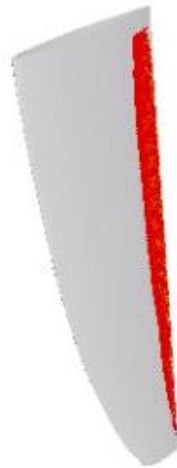
Figure 6.2: LSB at the Fin, Re: 5.0 \times 10^5 , 0^\circ AoA
