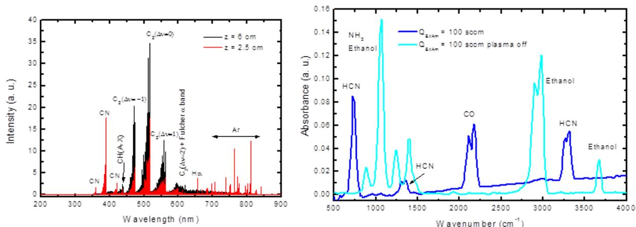
Figure 3 – (Left) OES spectrum from two different positions from the launcher ( $z = 2.5$  and  $6$  cm). (Right) FT-IR spectrum of the outlet gas stream with the plasma turned on and off. Both spectra were taken for the experimental conditions of sample NG<sub>3</sub>.
