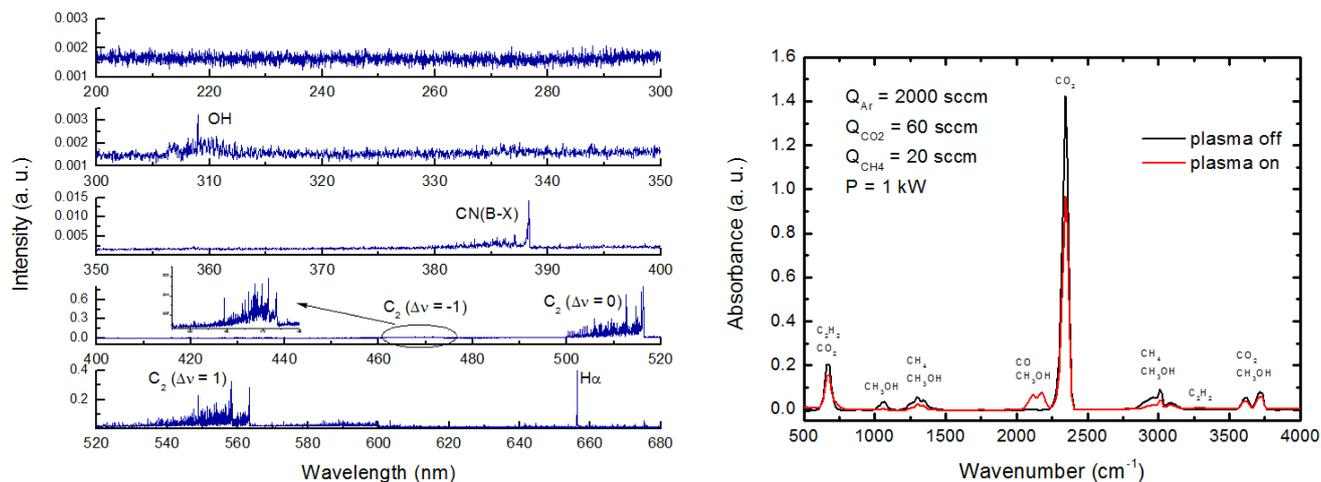
Figure 1 - (Left) OES spectrum from the region close the launcher, for the experimental conditions of sample ND2. (Right) FT-IR spectrum of the outlet gas stream with the plasma turned on and off, for the experimental conditions of sample ND1.
