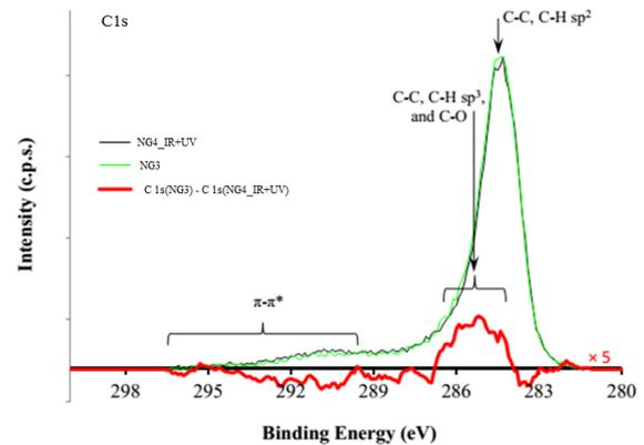
Figure 4 – (1<sup>st</sup>) SEM images from samples NG<sub>3</sub> (left) and NG<sub>4</sub>\_IR+UV (right). (2<sup>nd</sup>) Detailed XPS N1s regions of NG samples: a) NG<sub>4</sub>; b) NG<sub>4</sub>\_IR; c) NG<sub>4</sub>\_IR+UV. (3<sup>rd</sup>) Comparison between the C1s peaks for the samples NG<sub>3</sub> (green) and NG<sub>4</sub>\_IR+UV (black).
