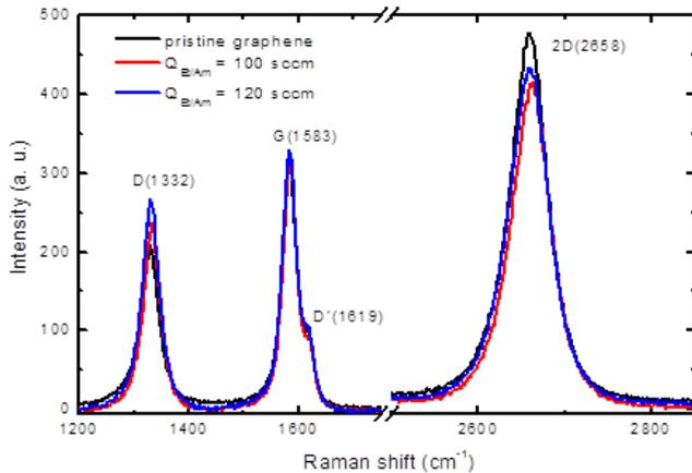
Figure 5 – (1<sup>st</sup>) 3D representation of the Raman spectrum taken from three different locations (sample NG<sub>4</sub>). (2<sup>nd</sup>) Raman spectrum for pristine graphene and samples NG<sub>3</sub> and NG<sub>4</sub>\_IR+UV.
