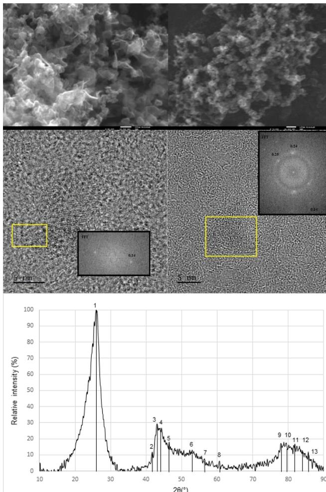
Figure 2 – (1<sup>st</sup>) SEM images of the samples ND1 (left) and ND2 (right). (2<sup>nd</sup>) HRTEM images of sample ND2. (3<sup>rd</sup>) XRD spectrum of sample ND2.
