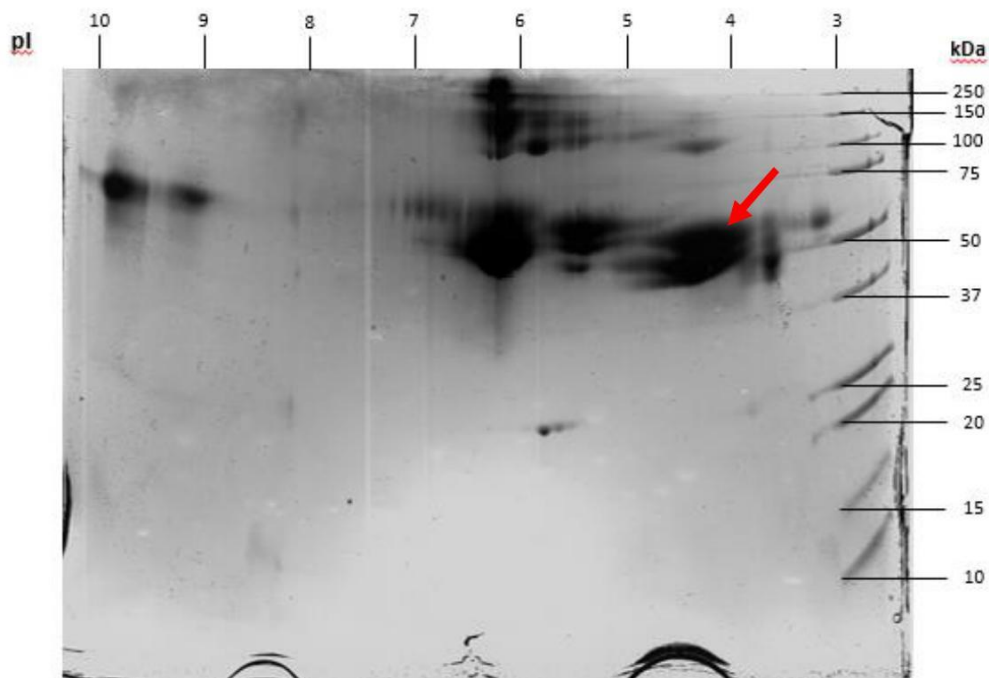
Figure 23 – Silver stained 2D-Electrophoresis a sample from the FT of the CHO DP-12 cell culture supernatant. Proteins (500µg) were precipitated and separated based on their pI in 7cm IPG strips (pH 3-10) and then applied on an SDS-PAGE gel. The red arrow points the most abundant protein present in the supernatant, BSA, which is added to the culture medium when adding the FBS.
