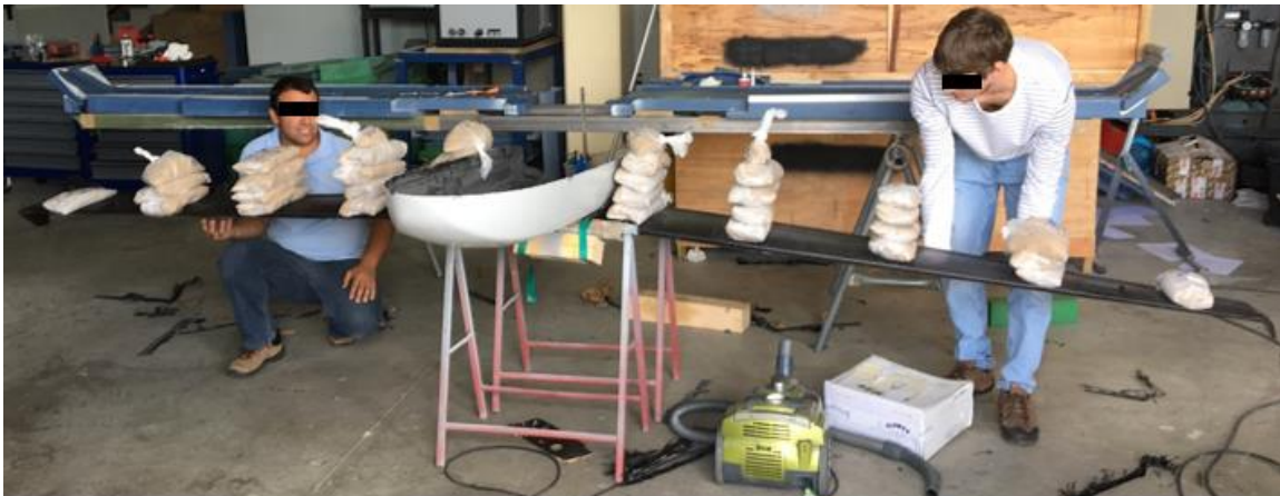
Figure 39 - UAV wing test (courtesy of "UAVision")
