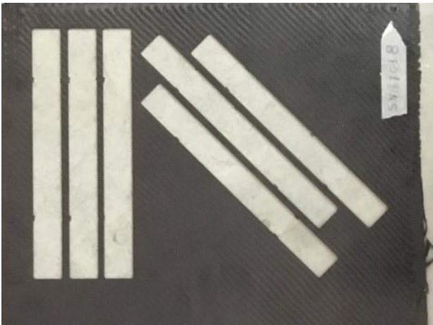
Figure 23 - Sheet of 2x2 twill weave carbon fibre (courtesy of “UAVision”)
