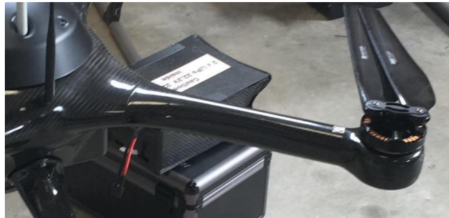
Figure 10 - Carbon-epoxy arm and rotor blades (courtesy of “UAVision”)
