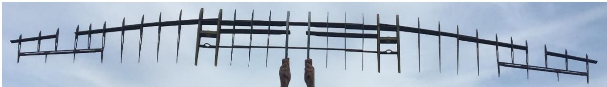
Figure 37 - Internal structure of the UAV wing tested (courtesy of “UAVision”)
