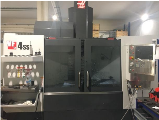
Figure 24 - Haas VF-4SS used to cut the specimens (courtesy of “UAVision”)
