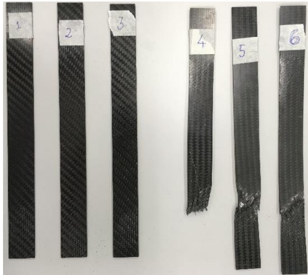
Figure 28 - Carbo-epoxy specimens after the tensile test (courtesy of “Técnico Lisboa”)
