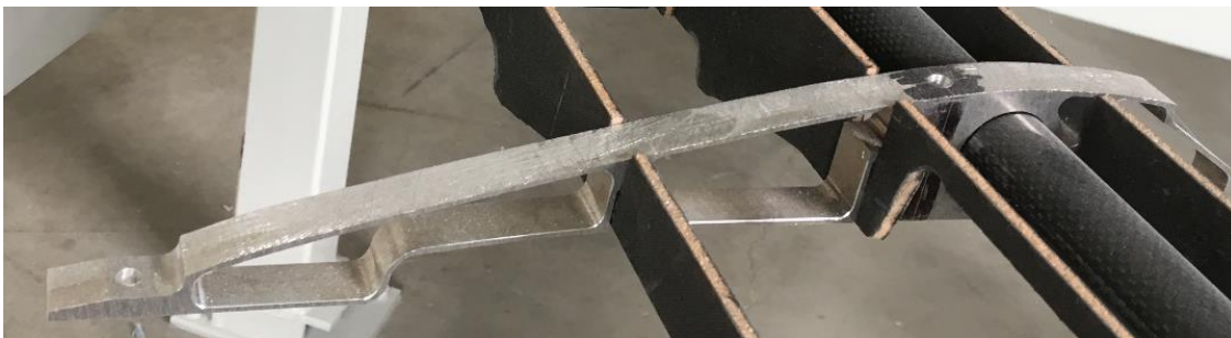
Figure 43 - Aluminum rib in the real wing (courtesy of UAVision)
