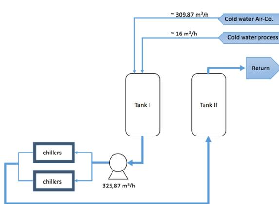
Figure 3. Cooling system that serves the factory and the air-conditioning equipment
