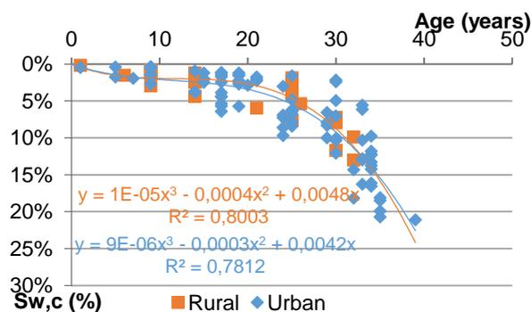
**Figure 11 - Degradation curve of the aluminium framework, according to the surrounding environment**
