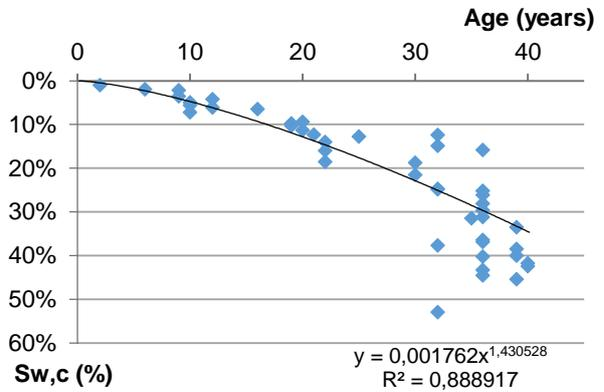
**Figure 4 - Degradation curve of the 45 wooden frameworks analysed in the fieldwork**
