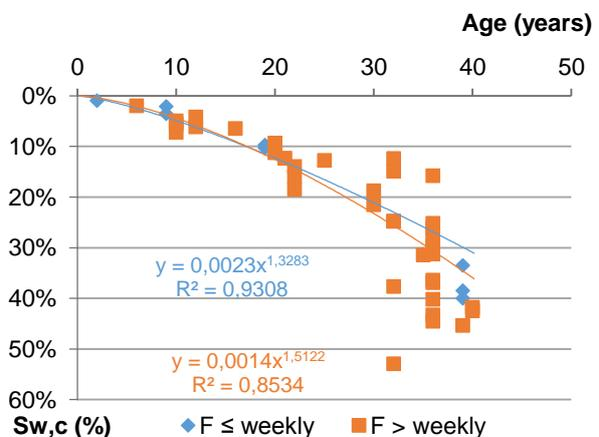
**Figure 6 - Degradation curve of the wooden framework, according to the frequency of cleaning actions**
