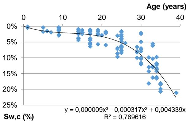
**Figure 3 - Degradation curve of the 112 aluminium frameworks analysed in the fieldwork**
