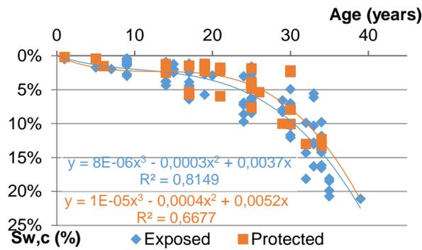
**Figure 7 - Degradation curve of the aluminium framework, according to the window span exposure**
