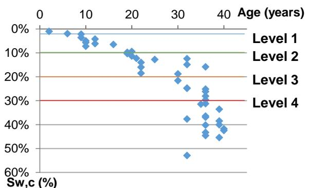
**Figure 2 - Degradation severity of wooden framework inspected during the fieldwork**
