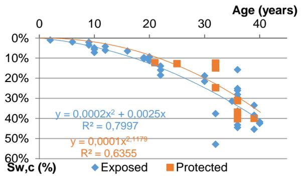
**Figure 8 - Degradation curve of the wooden framework, according to the window span exposure**
