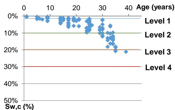
**Figure 1 - Degradation severity of aluminium framework inspected during the fieldwork**
