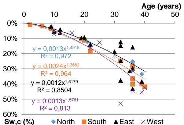
**Figure 10 - Degradation curve of the wooden framework, according to window span orientation**
