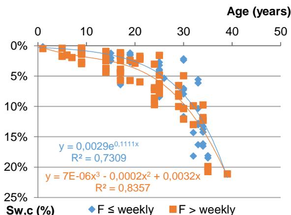
**Figure 5 - Degradation curves of the aluminium framework, according to the frequency of cleaning actions**
