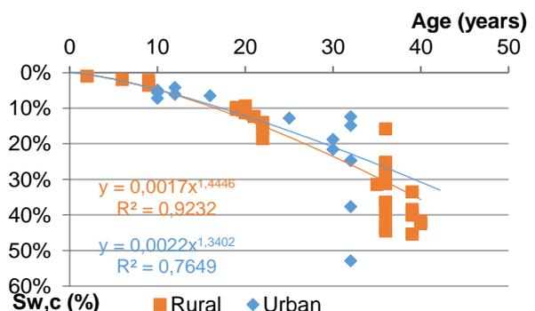
**Figure 12 - Degradation curve of the wooden framework, according to the surrounding environment**
