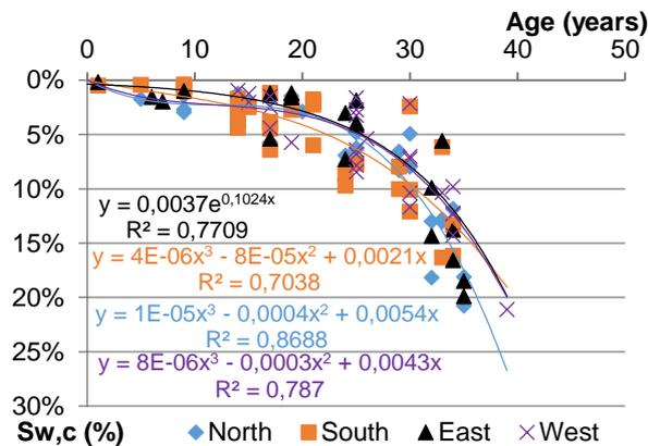
**Figure 9 - Degradation curve of the aluminium framework, according to window span orientation**
