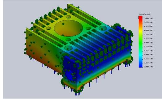
Figure 6 Cooling base under thermal stress
