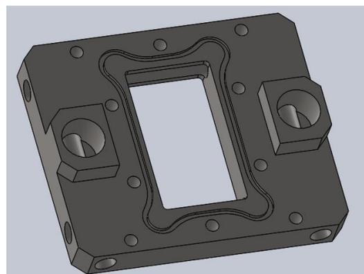
Figure 10 Probe housing for the 5 MHz probe
