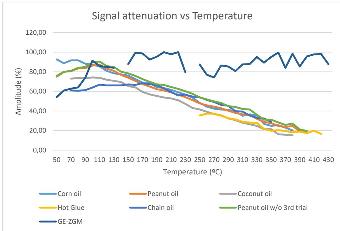
Figure 15 Signal attenuation of longitudinal waves of all tested couplants
