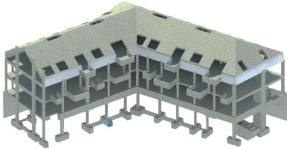
Figure 3 - Perspective of the finished 3D structural model on Revit
