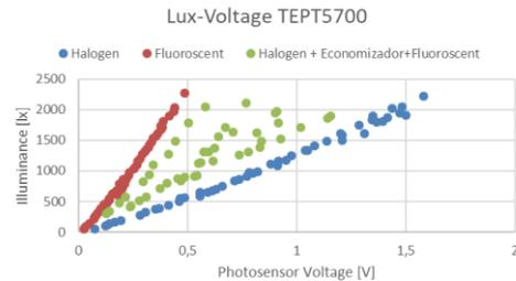
Figure 4 – Lux-Voltage Relation for TEPT5700 circuit. This shows the TEPT 5700 circuit voltage acquired with the ADC for different light types.
