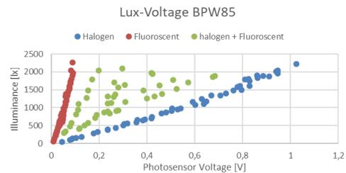
Figure 5 - Lux-Voltage Relation for BPW 85 circuit. This shows the TEPT 5700 circuit voltage acquired with the ADC for different light types.
