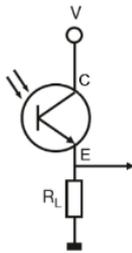
Figure 2 - Phototransistor in a common collector topology.
