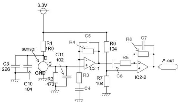
Figure 6 – Schematic for applying a PIR sensor as a motion detector [5].
