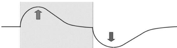
Figure 7 – PIR sensor - output voltage representation [9].
