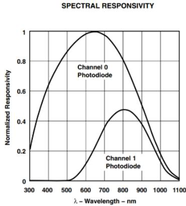
Figure 1- TSL 2561 – Photoelements spectral responsivity.
