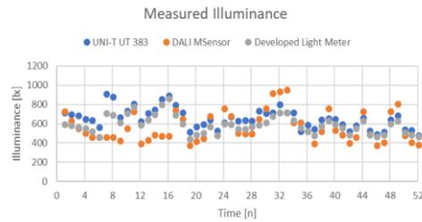
Figure 9 – Representation of measures made with the developed light meter, UNI-T UT 383 and the DALI MSensor.
