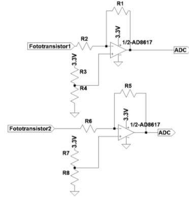
Figure 3 – Topology for amplifying the output signal of the circuit present in Figure 2.
