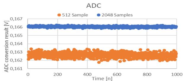
Figure 8 – AD7091R-5 - Result for 1000 conversions of two different DC, these voltages were acquired with a different number of samples per acquisition.
