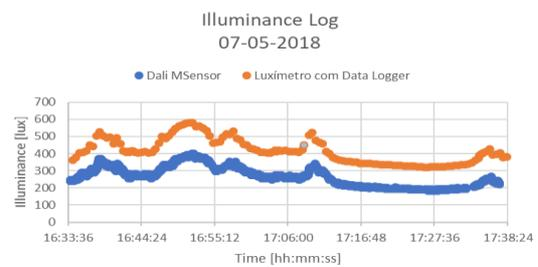
Figure 10 – Results for illuminance measures along time for the DALI MSensor and the developed light meter.
