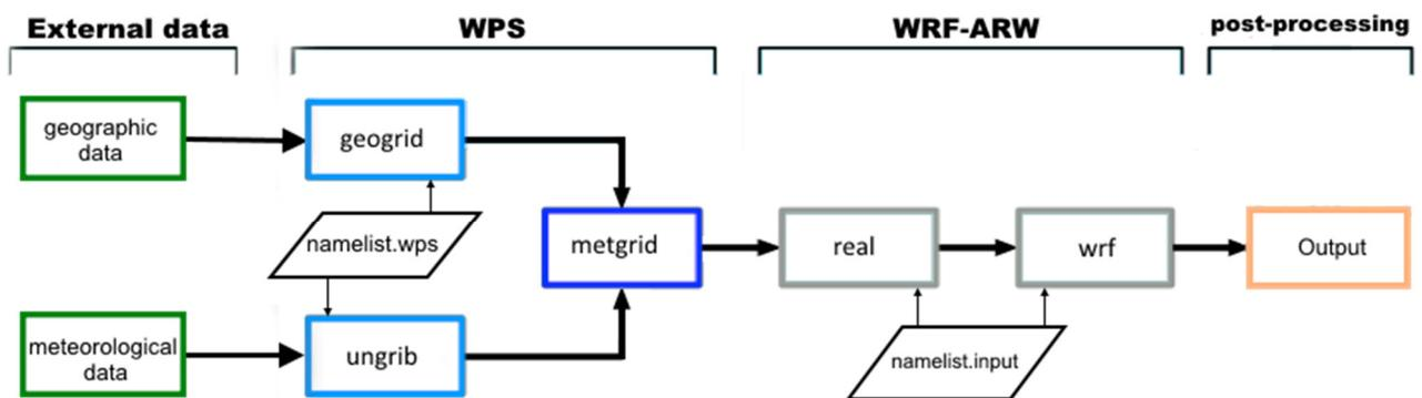
Figure 1 - WRF model data flow
