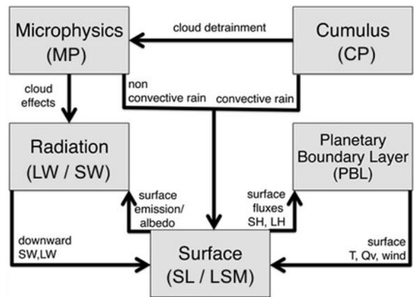
Figure 4 – Physical parameterizations interactions in WRF model
