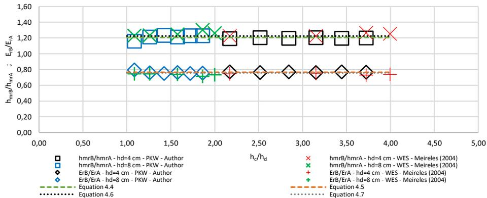
Figure 10 – Influence of applying hypothesis A or B on the equivalent clear water depth and residual specific energy.
