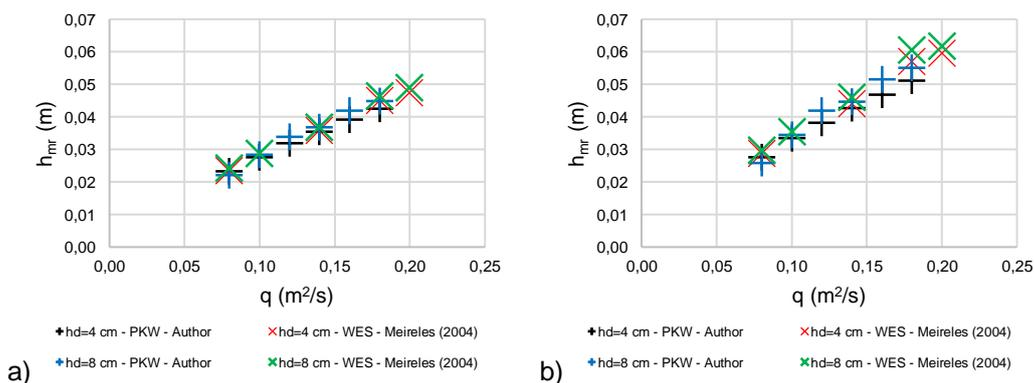
Figure 9 – Equivalent clear water depth at the upstream section of the hydraulic jump: a) hypothesis A; b) hypothesis B.
