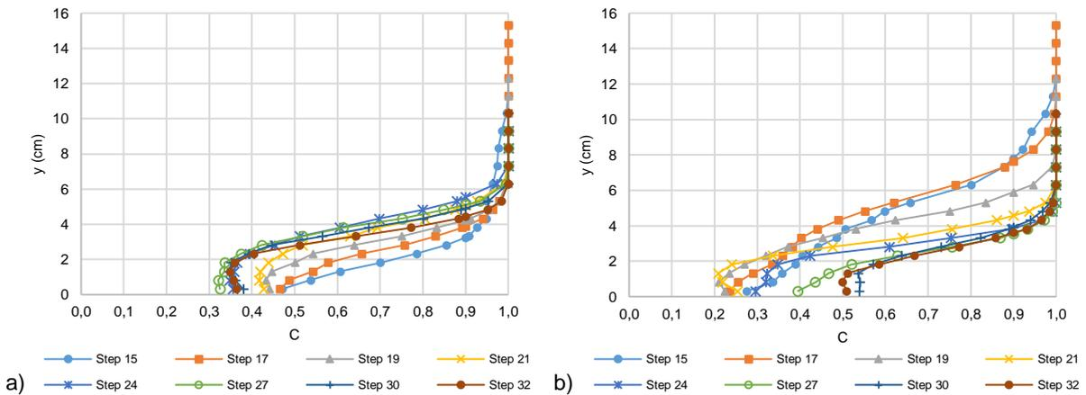
Figure 2 – Air concentration distribution along the chute 4 cm high steps, for  $Q=80$  l/s: a) in the symmetry axis of the outlet key; b) in the symmetry axis of the inlet key.
