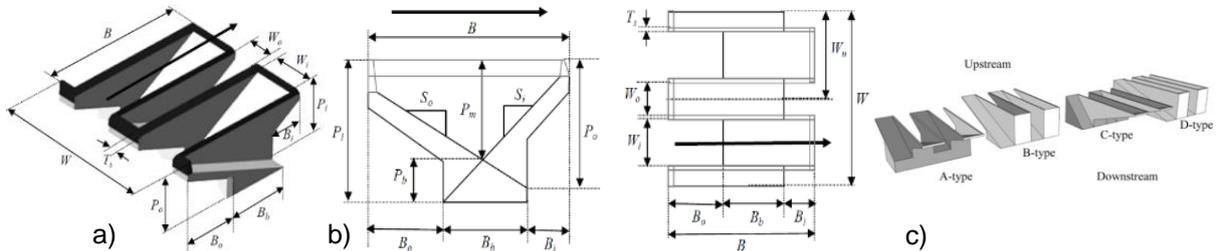
Figure 1 – Representation of a PKW weir: a) 3D view; b) top and side views c) four types of PKW (Pralong et al., 2011, Ercicum et al., 2017).
