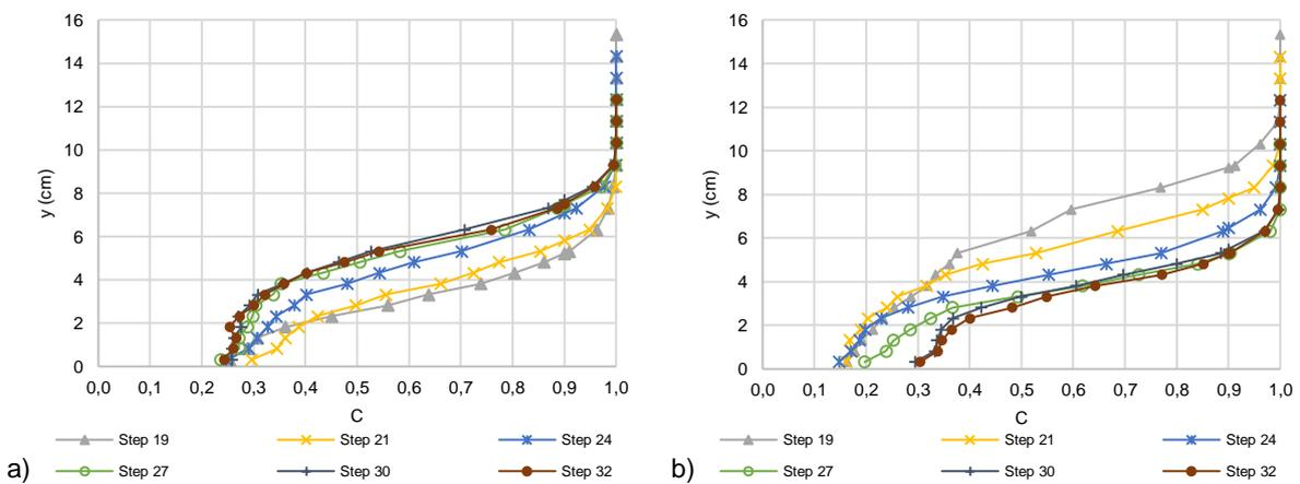
Figure 3 – Air concentration distribution along the chute with 4 cm high steps, for  $Q=140$  l/s: a) in the symmetry axis of the outlet key; b) in the symmetry axis of the inlet key.
