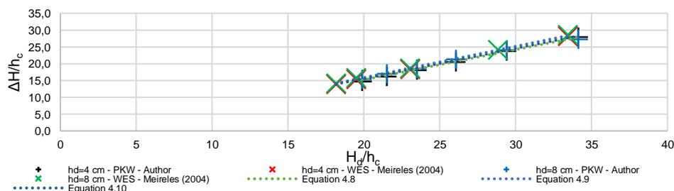
Figure 11 – Dimensionless energy dissipation at the spillway in function to the relative dam height (hypothesis B).
