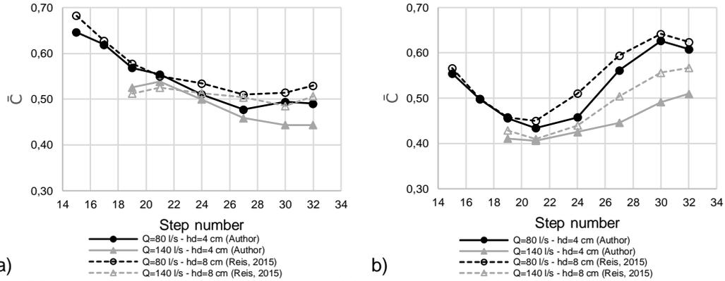
Figure 4 – Mean air concentration along the chute: a) in the symmetry axis of the outlet key; b) in the symmetry axis of the inlet key.
