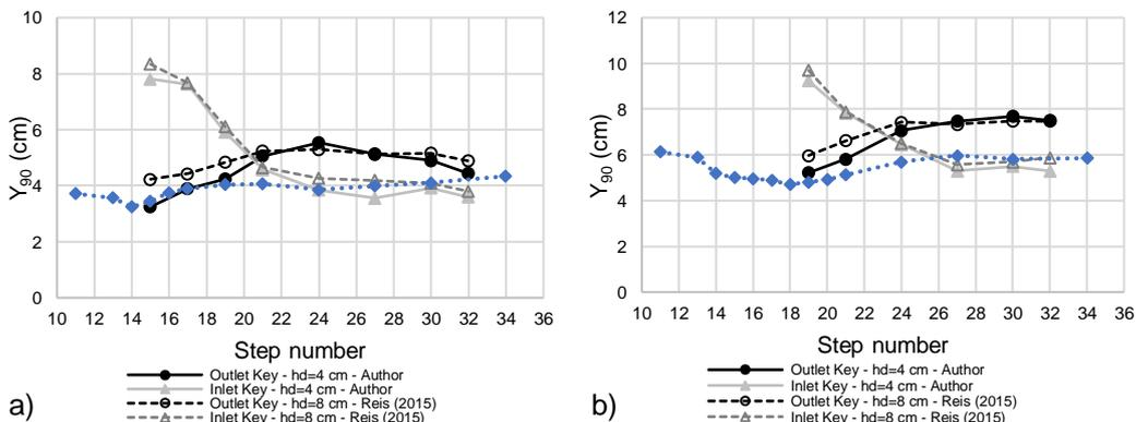
Figure 7 – Characteristic flow depth  $Y_{90}$  along the chute, in the symmetry axes of the inlet and outlet keys: a) Q=80 l/s; b) Q=140 l/s.
