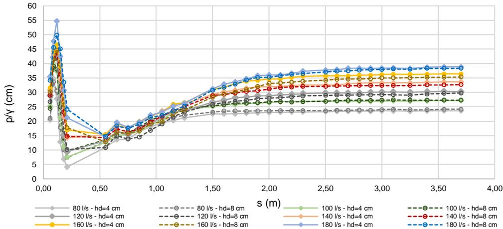
Figure 8 – Piezometric heads along the stilling basin with the hydraulic jump starting at the impact point of the flow in the stilling basin.
