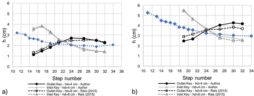
Figure 6 – Equivalent clear water depth along the chute, in the symmetry axes of the inlet and outlet keys: a) Q=80 l/s; b) Q=140 l/s.
