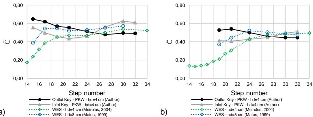
Figure 5 – Mean air concentration along the chute, in the symmetry axes of the outlet and inlet keys: a)  $Q=80$  l/s; b)  $Q=140$  l/s.
