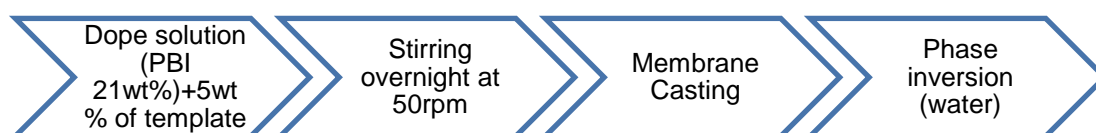
Fig. 14- Process of phase inversion for membrane fabrication
