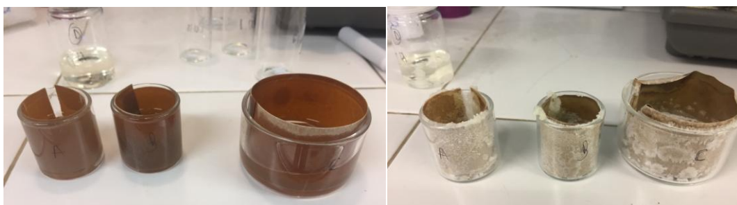
Fig. 40- Illustration of recrystallization on membrane: membrane in contact with solution (left); formation of crystals (right)
