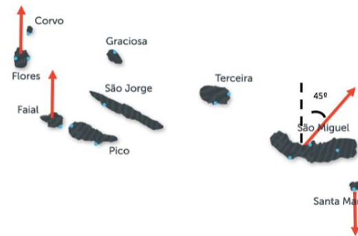
Figure 10: Direction of maximum propagation of the 18 elements' Yagi antennas in the GSs (adapted from [15]).
