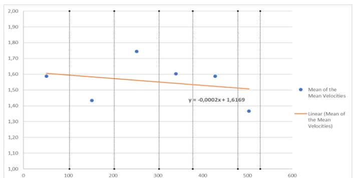
Figure 5 - Mean of the average velocities in each of the drilling stages and respective trend line.
