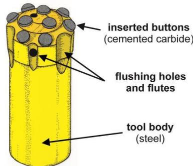
Figure 2 - Drilling bit and its constituents (Source Plinninger, 2008).
