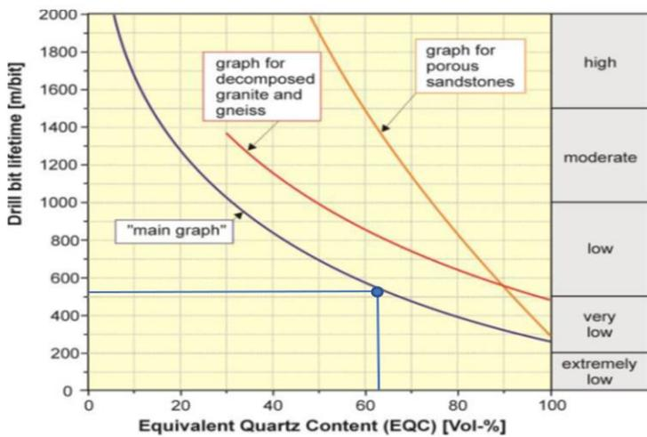
Figure 10 - Correlation between EQC and the average bit lifetime.
