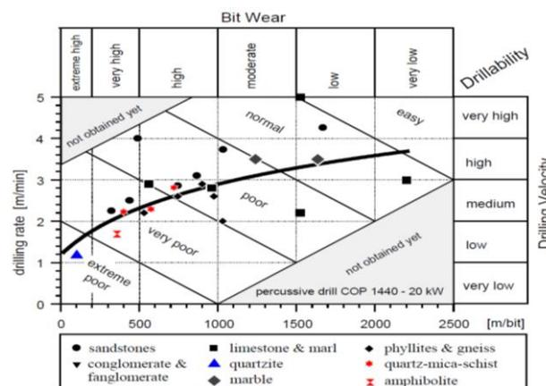
Figure 1 - Drillability classification diagram (Source: Thuro, 1997b).
