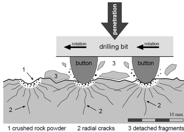
Figure 3 - Drilling Process (Source: Thuro & Spaun, 1996).
