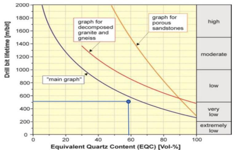
Figure 11 - Correlation between EQC, calculated from its correlation with CAI, and the average bit lifetime
