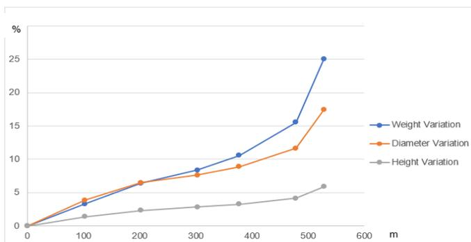
Figure 4 - Percentage variation of average loss of weight, diameter and height of the bits along the drilled meters.
