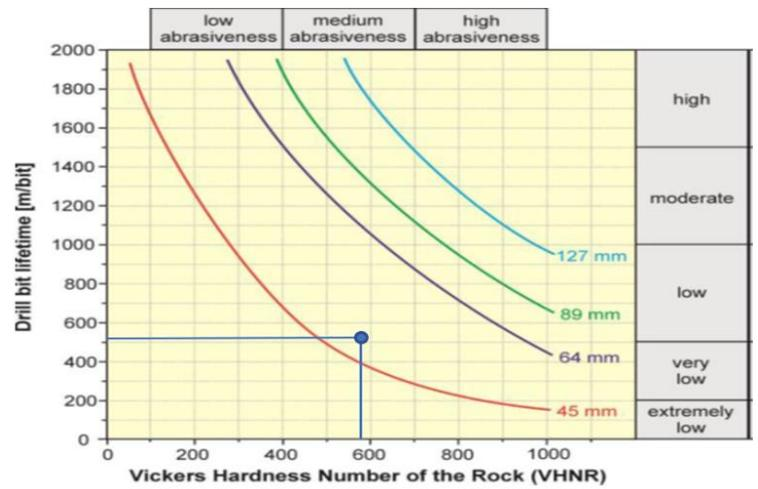
Figure 9 - Correlation between VHNR, calculated from its correlation with CAI, and the average bit lifetime.
