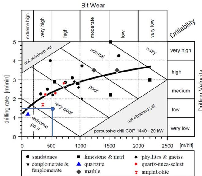
Figure 14 - Point obtained in the drillability classification diagram.
