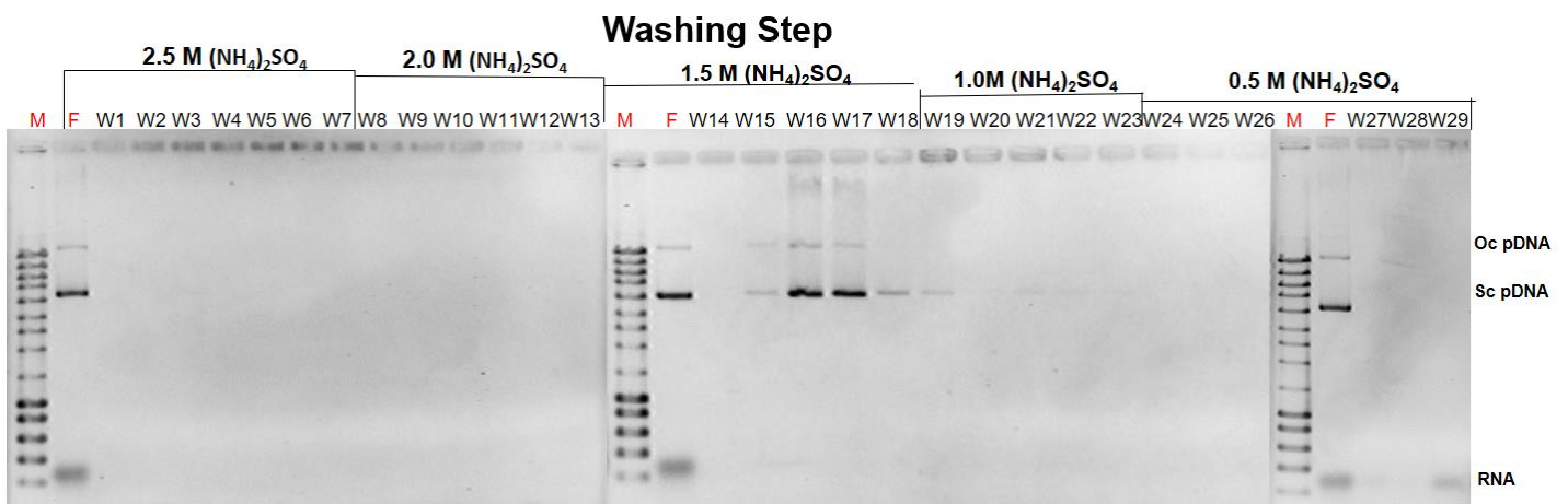
Figure A11: Gel electrophoresis obtained from the bench chromatographic assay using 1 mL of Sepharose CL-6B derivatized with ligand 0/0 packed in a column in 4 mL hydrophobic conditions (stepwise washing/elution from 0.5 M to 2.5 M (NH 4 ) 2 SO 4 ). a) Fractions collected during washing step; W1 to W29- Fractions collected, in increasing order, during washing step, where the concentration of elution buffer was decreased from 2.5 M to 0.5 M (NH 4 ) 2 SO 4 ; M- DNA Ladder III (NZYtech); F- Feed (clarified lysate added to the column); sc- Supercoiled; Oc- open circular. Complete band size description of DNA ladder is presented in appendix II.
