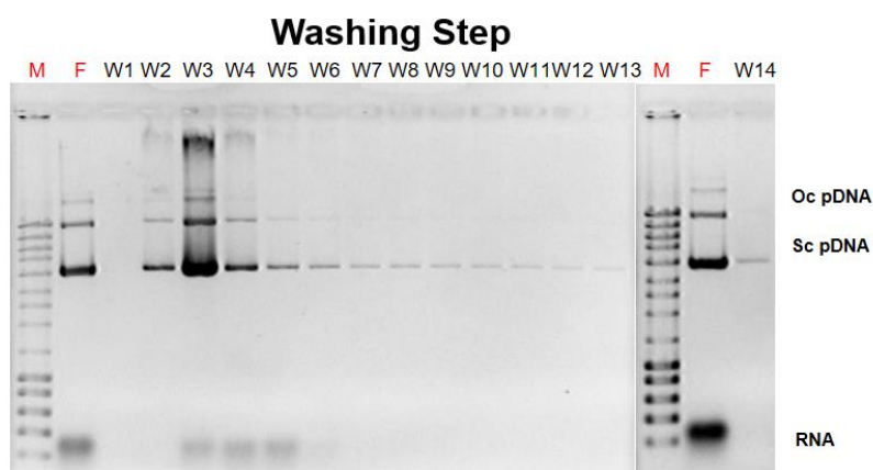
Figure A9: Gel electrophoresis obtained from the bench chromatographic assay using 1 mL of Sepharose CL-6B derivatized with ligand 0/0 packed in a 4 mL column and evaluated in hydrophilic conditions. W1 to W14- Fractions collected, in increasing order, during washing, using Tris-HCl 20 mM, pH 8.0; M- DNA Ladder III (NZYtech); F- Feed (clarified lysate added to the column); sc- Supercoiled; oc-open-circular. Complete band size description of DNA ladder is presented in appendix II.
