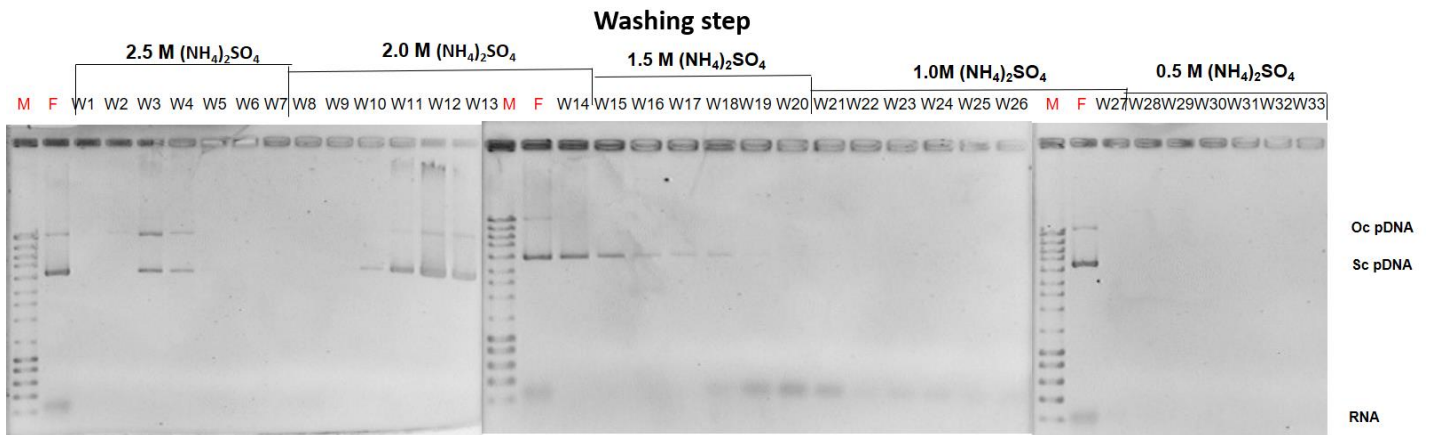
Figure 19: Gel electrophoresis obtained from the bench chromatographic assay using 1 mL of Aminated Sepharose Cl-6B packed in a 4 mL column in hydrophobic conditions (stepwise washing/ elution from 2.5 M to 0.5 M (NH 4 ) 2 SO 4 ). a) Fractions collected during washing step; W1 to W33- Fractions collected, in increasing order, during washing step, where the concentration of washing buffer was decreased from 2.5 M to 0.5 M (NH 4 ) 2 SO 4 ; M- DNA Ladder III (NZYtech); F- Feed (clarified lysate added to the column); sc- Supercoiled; Oc- open-circular. Complete band size description of DNA ladder is presented in appendix II.
