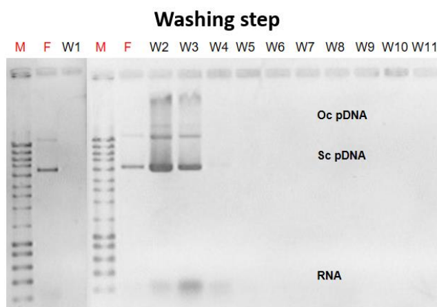
Figure 21: Gel electrophoresis obtained from the bench chromatographic assay using 1 mL of Aminated Sepharose CL-6B actiated with cyanuric chloride packed in a 4 mL column in hydrophilic conditions. W1 to W11- Fractions collected, in increasing order, during washing, using Tris-HCl 20 mM, pH 8.0; M- DNA Ladder III (NZYtech); F- Feed (clarified lysate added to the column); sc- Supercoiled; Oc- open-circular. Complete band size description of DNA ladder is presented in appendix II.
