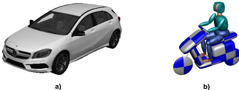
Figure 3.34 - a) car , modelb) multibody model of the scooter and driver used in crash simulations.
