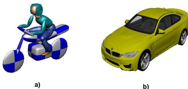
Figure 3.32 - a) multibody model of the motorcycle and driver, b) model of the car used in crash simulations.
