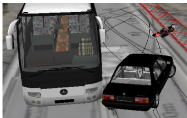
t = 0,950s – Point of impact of the second collision
