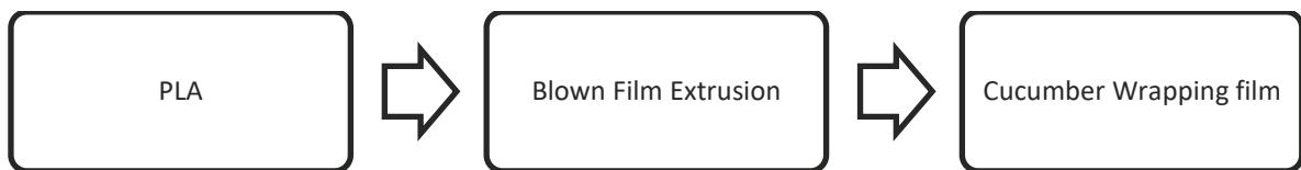
Figure 16 - Cucumber wrapping film manufacturing process.
