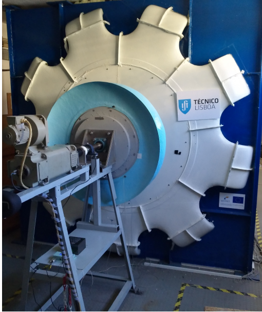
Fig. 12: Layout of the test rig, showing the electrical motor/generator, the inlet duct and the manifold.
