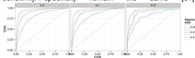
**Figure 5:** ROC curves for models tested with 3 different data sets with ratios positive/negative varying from 0.4, 0.1 to 0.01 [32].
