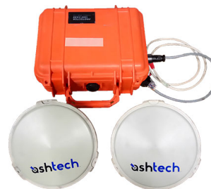
Figure 6.5: DGPS acquisition system. Two antennas and the logging and supply system.
