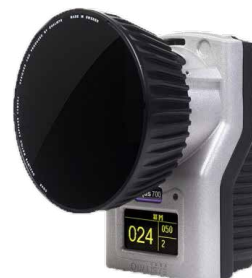
Figure 5.3: Infra-red camera used by Qualisys software to acquire the vehicle position
