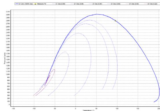
Figure 3 Phase envelope for recombined samples
