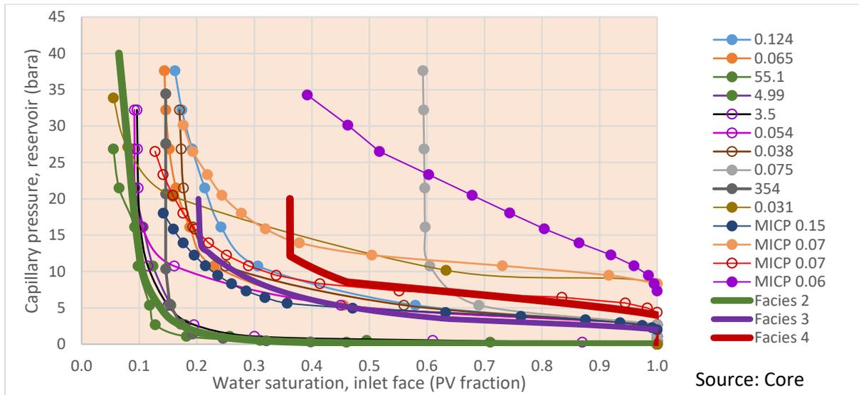
Figure 2 Capillary Pressure Curves – each curve is the capillary pressure curve of a different core
