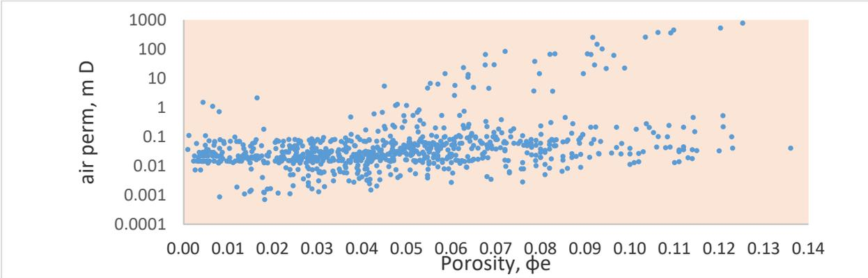
Figure 1 Relationship of permeability to porosity
