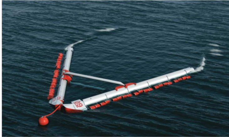
Figura 15- Overtopping Wave Dragon.
