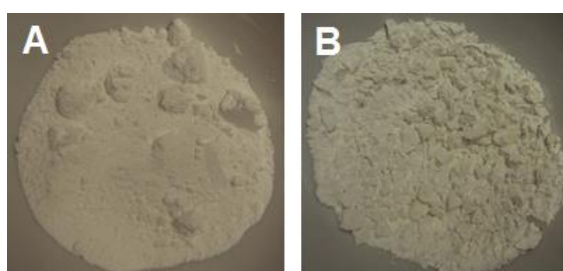
Figure 3-3 – ZSM-5 zeolite after calcination: A) zeolite without silver; B) zeolite with embedded silver.
