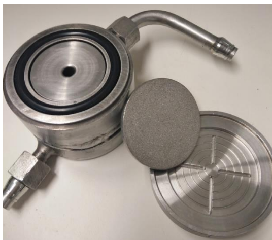
Figure 3-11 – Permeation cell used in ultra and nanofiltration installations.
