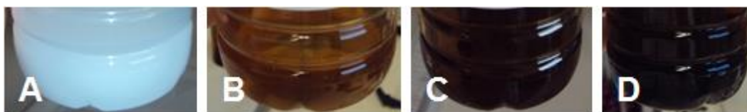
Figure 3-5 – Comparison of the casting solutions with zeolite and silver loaded zeolite with A: 0%; B: 0,005%; C: 0,03% and D: 0,07% of silver in the casting solution.
