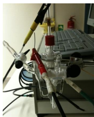
Figure 3-23 – Electrochemical cell used to study the electrochemical behaviour of silver entrapped inside zeolites.
