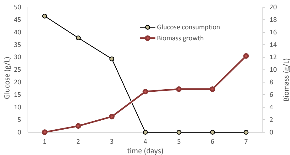
Figure 15 – Biomass growth and glucose consumption curves for a no-feed situation.
