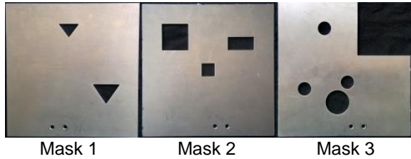
Figure 12: Masks used in the experiments to create different illumination patterns on the cell
