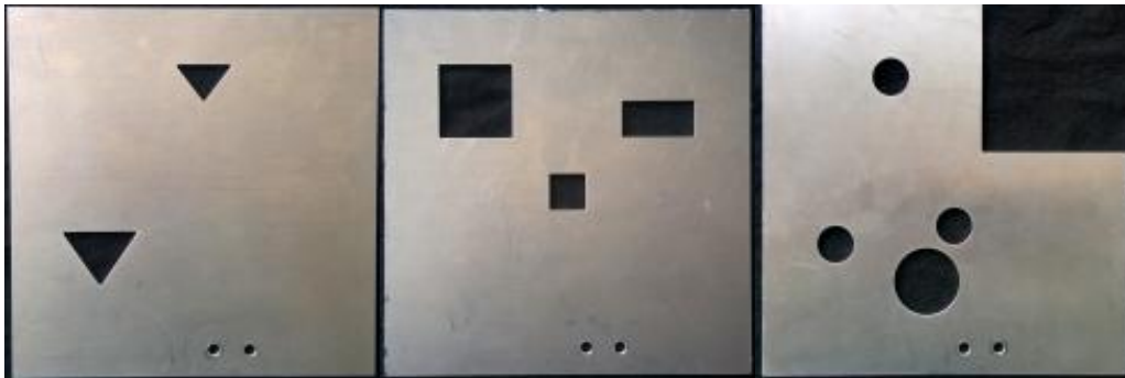
(a) masks used to create different illumination profile on cell surface
