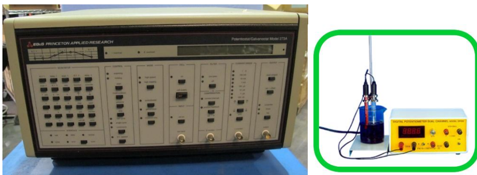
Fig. 4 – Potentiostat/Galvanostat Princeton Applied Research/EG&G Model 273A (left) and Digital Potentiometer Dual Channel model DP002 (right).
