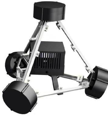
Figure 1.2: Reaction Wheel regular tetrahedral configuration (obtained from ESA reports)
