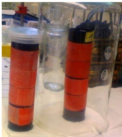
Figure 12: small scale sedimentation tower (tower height of 20 cm)
