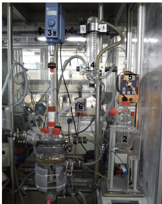
Figure 18: Polymerization unit. 1-Reactor, 2- Pré-emulsion tank, 3-Stirrer+impeller, 4-Condenser, 5-Pump responsible for forwarding the pre emulsion to the reactor, 6- Pump responsible for forwarding the water from the bath to the reactor jacket.
