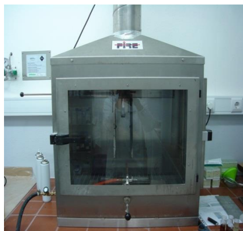
Figure 1. Chamber for the fire resistance test.
