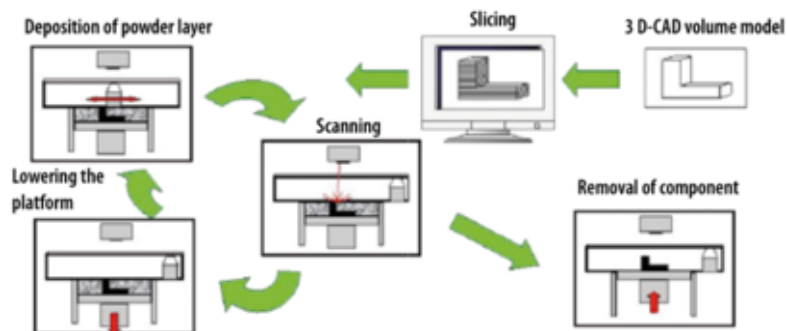
Figure 2.19 - Selective laser melting process [46].
