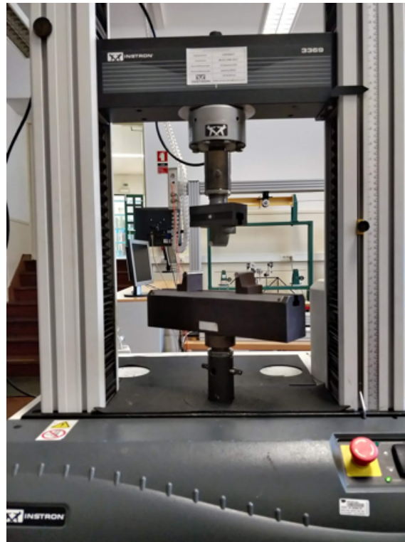
Figure 3.14 - Instron 3369 testing machine present at the IST Experimental Mechanics Laboratory .
