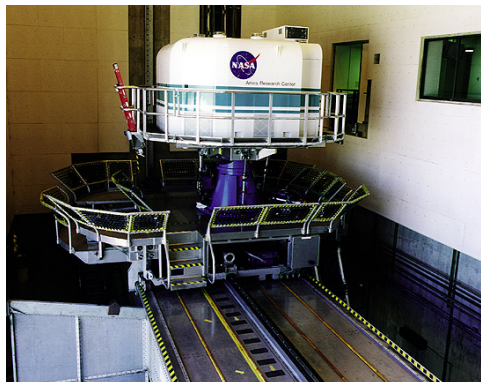
Figure 2.1: VMS, simulator build by NASA in Ames, California USA
