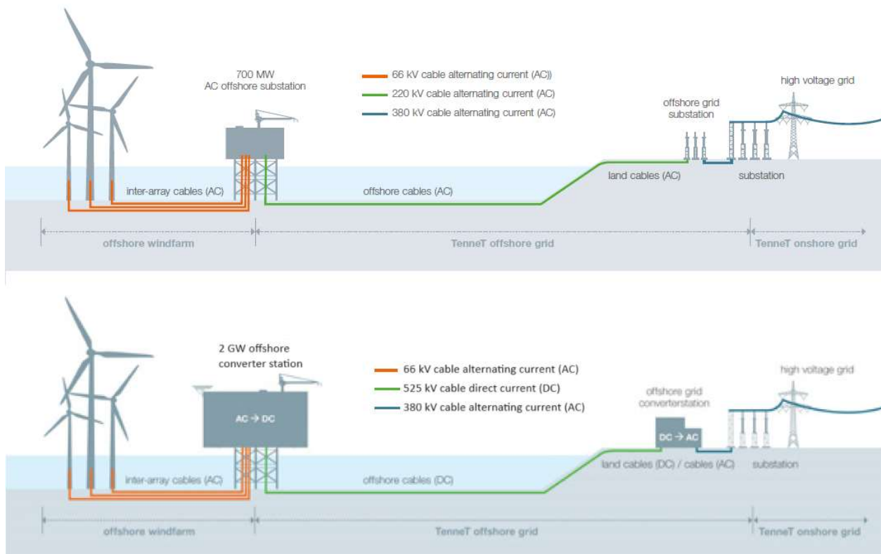
Figure 8: Depiction of the systems connecting an offshore wind farm to the onshore grid. Dutch TSO TenneT is responsible for the segments from the offshore substation through to the onshore grid. Source: [1]
