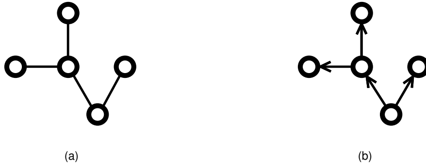
Figure 2.1: Two examples of networks, where nodes are represented by circles and edges are the lines between them: (a) is a network with undirected edges and (b) has directed edges.
