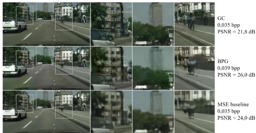
Figure 19 - Evaluation between GC, BPG and MSE baseline using an image from the Cityscapes dataset (Adapted from [30]).
