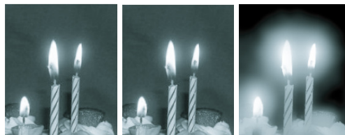
Figure 2.6: First image is the image to be denoised (image I ), the second image is the one containing the edges we wish to preserve (Image E ) and the last one is the result of the cross bilateral filter [14].
