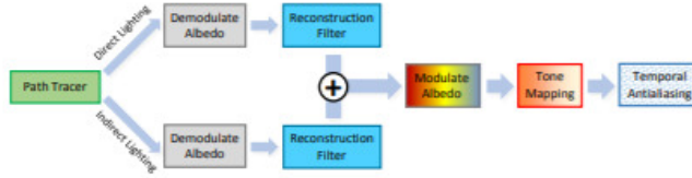
Figure 2.8: High level view of SVGF pipeline [16]
