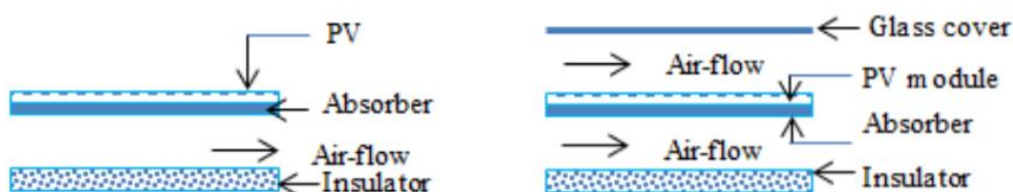
Figure 5.1 Cross-section of a single pass PV/T air collector (left) and a double pass PV/T air collector (right) [29]
