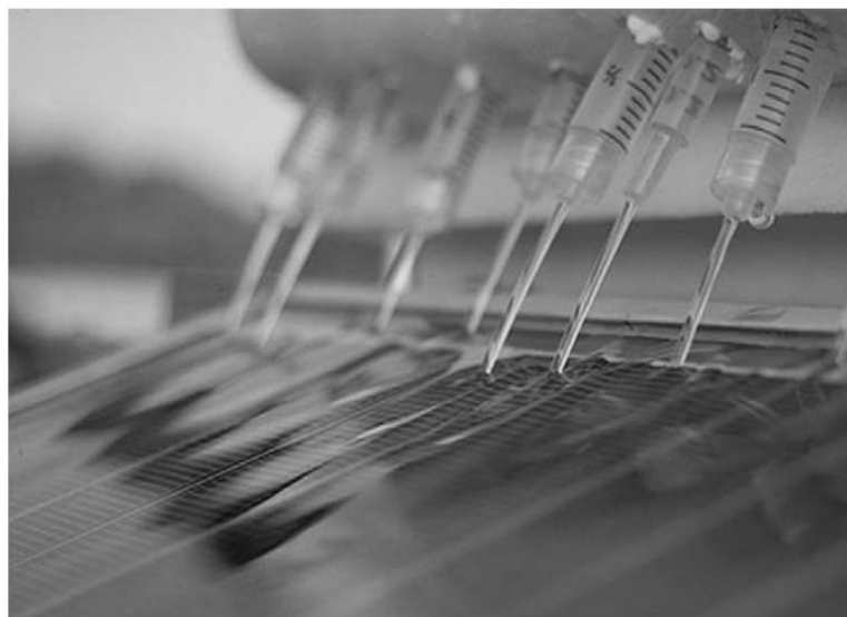
Figure 5.5 Creation of the thin film of water over the PV module by a series of nozzles [35]
