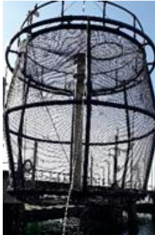
Fig. 9 – Prototype of a semi-submersible cage of the Cage4PtSea project Fonte: Cage4PtSea project
