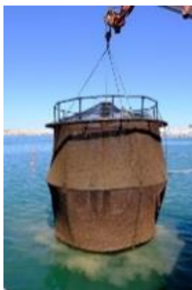
Fig. 10 – Cage when it left the sea after a stay of 6 months Fonte: Cage4PtSea project
