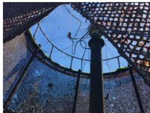
Fig. 12 – Stretchers in the upper zone after staying at sea for 6 months Fonte: Cage4PtSea project
