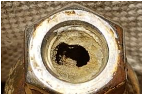
Fig. 17 - Fractured screw inside the nut Fonte: Cage4PtSea project. Ferreira A,
