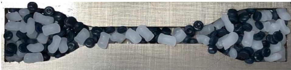
Figure 3.7. Difference in size and geometry of the rHDPE (blue) and vHDPE (white) pellets inside the mold
