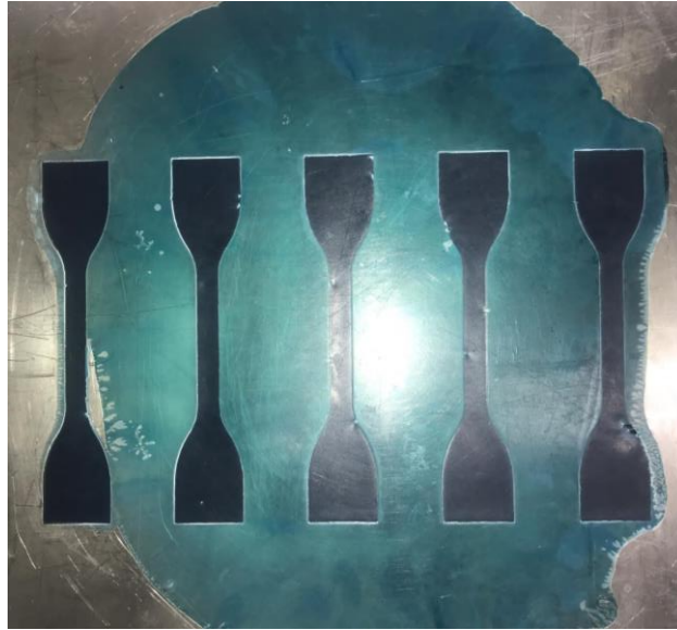
Figure 4.3. Specimens of 100% rPP when the mold was overfilled.
