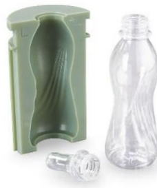
Figure 2.17. A mold for a plastic bottle, a parison or preform and the final plastic bottle obtained through blow molding
