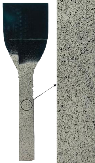
Figure 3.3. Painted test specimen (a) and detail of the painted pattern (b)
