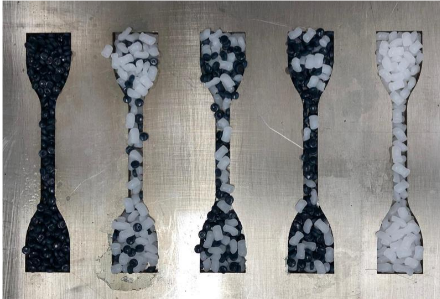
Figure 3.10. Mold prefilled with mixtures of recycled and virgin HDPE: 100% rHDPE, 25% rHDPE, 50% rHDPE, 75% rHDPE and 0% rHDPE
