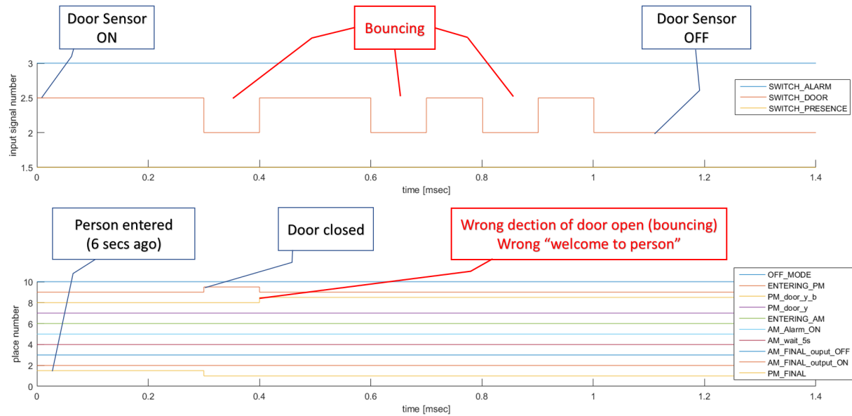
Figure 5.13: Behaviour of Petri net’s region of Figure 5.9 given table U_t (5.5).
