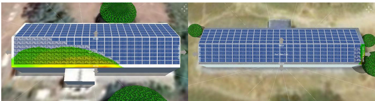
Figure 3.6. PVSOL shading analysis of VC Building Southern Façade (left) and Lecturers' Building Eastern Façade (right).
