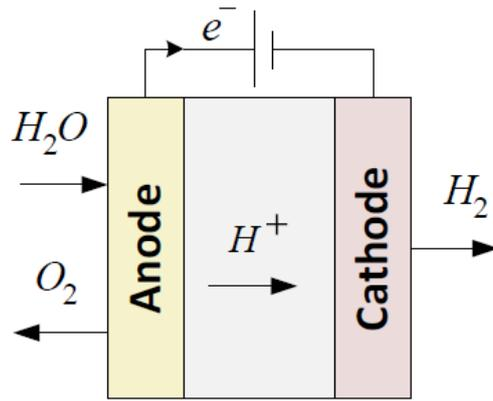
Figure 23 PEM electrolysis process illustration [16]
