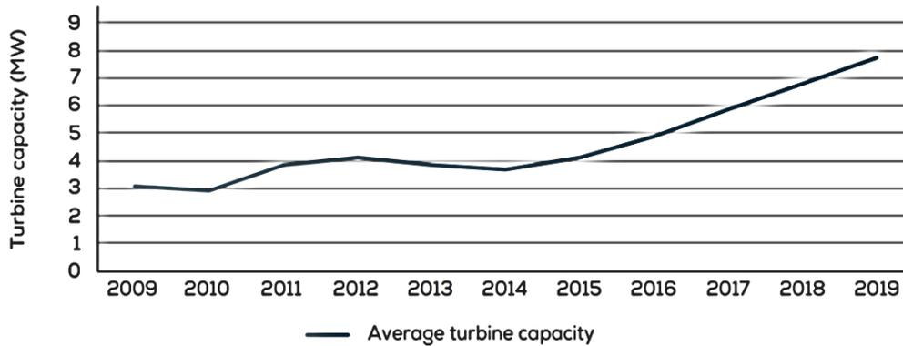
Figure 10 Average capacity per installed turbine [32]
