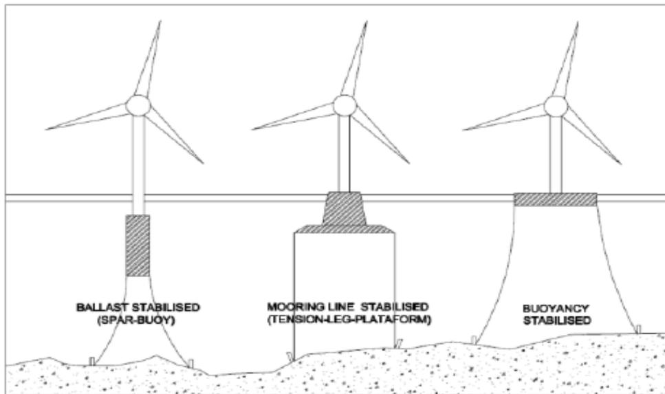
Figure 13 Floating wind structures [36]
