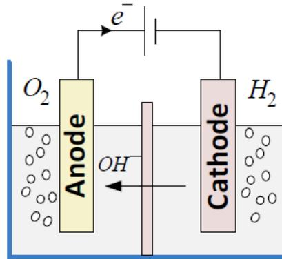
Figure 22 Alkaline electrolysis process illustration [16]
