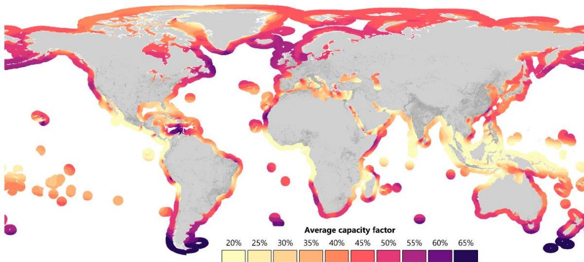
Figure 6 Average simulated capacity factors for offshore wind worldwide [17]
