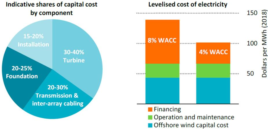
Figure 1 Offshore wind initial investment breakdown by component and LCOE for projects completed in 2018 [17]
