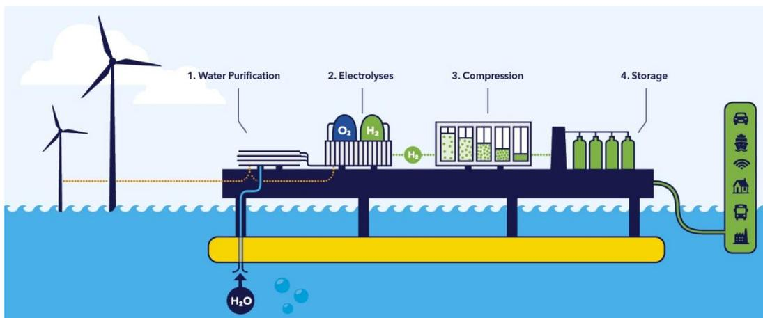
Figure 25 Offshore  $H_2$  plant configuration [59]
