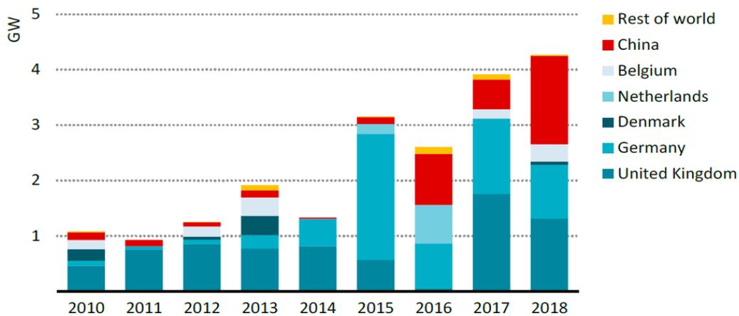
Figure 4 Annual offshore wind capacity additions by region [17]
