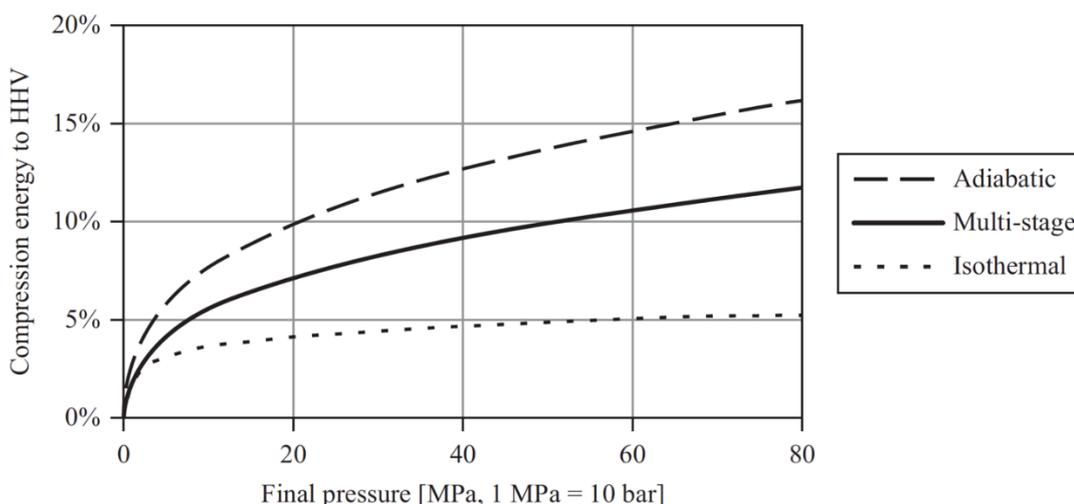
Figure 29 Energy required to compress H<sub>2</sub> in terms of its HHV
