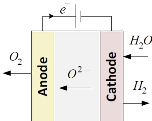
Figure 24 SOE process illustration [16]
