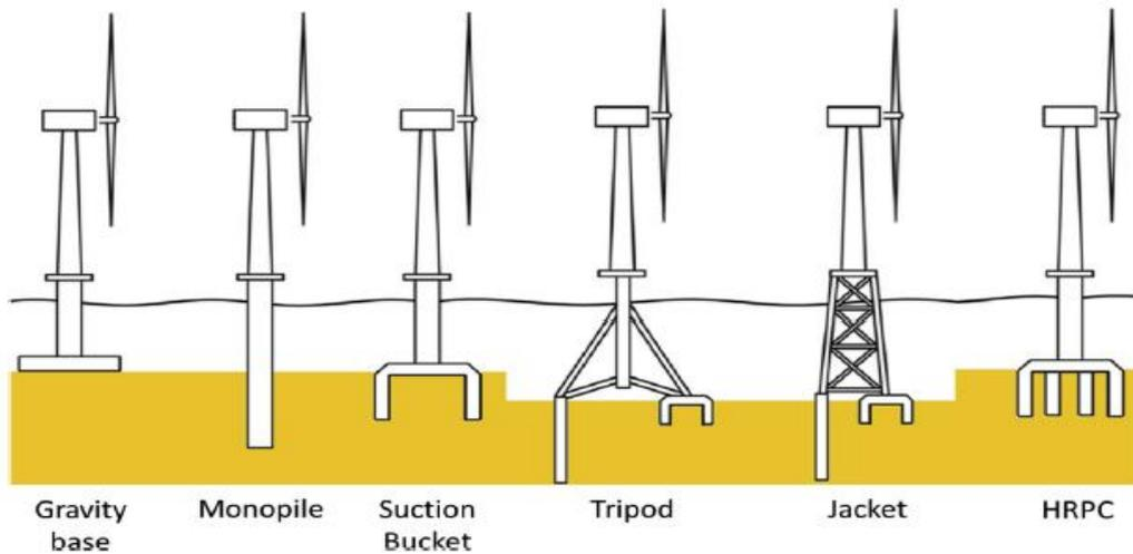
Figure 12 Most common offshore wind turbines structures [22]
