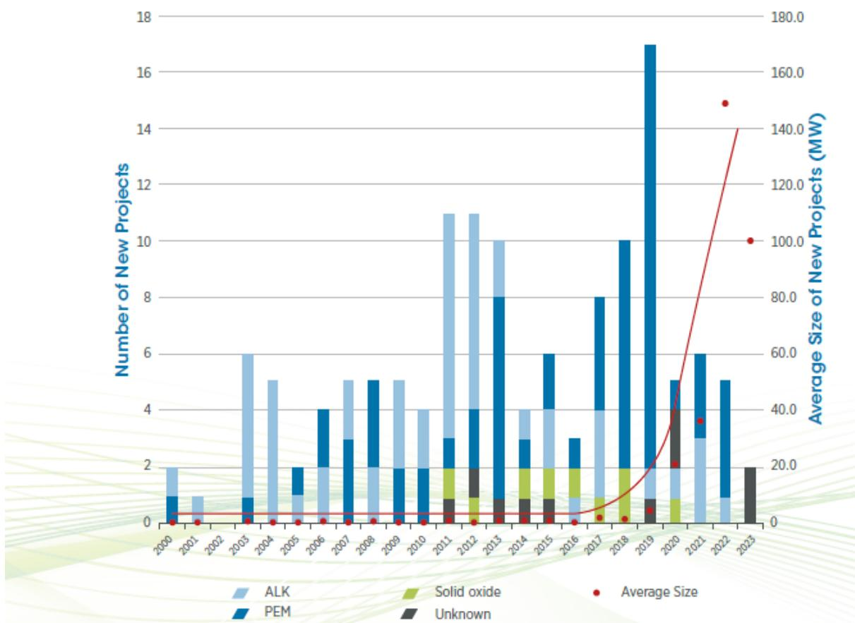
Figure 20 Timeline of power-to-H<sub>2</sub> projects by electrolyser technology and project scale [51]
