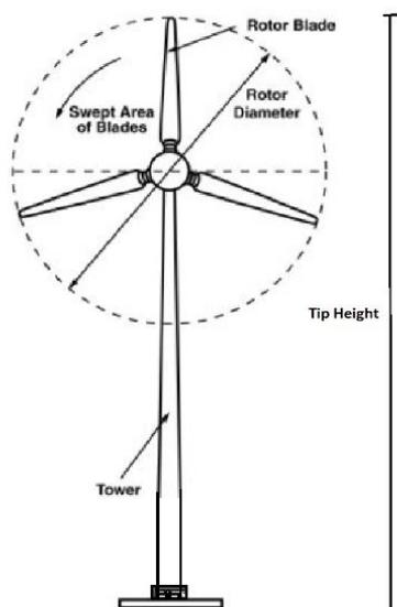
Figure 9 Wind turbine tip height and swept area [33]
