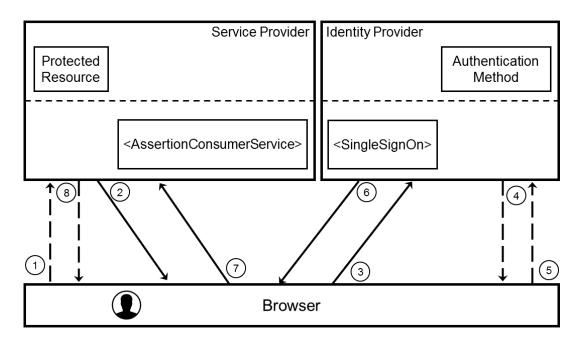
Figure 2.1: SAML Authentication Process using POST->POST Profile
