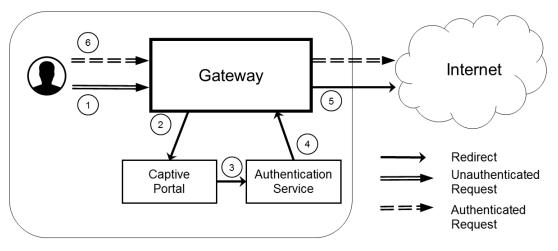
Figure 2.2: Example of a System with an integrated Captive Portal and Authentication Service (AS)
