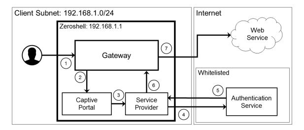
Figure 4.18: eAccess Authentication flow using Zeroshell's Captive Portal with external SAML authentication
