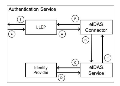
Figure 4.19: eAccess' AS individual components and authentication flow
