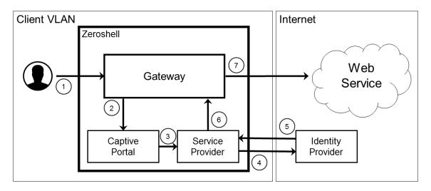
Figure 3.5: Authentication Flow in a Zeroshell system using it's Shibboleth Service Provider and an external Identity Provider
