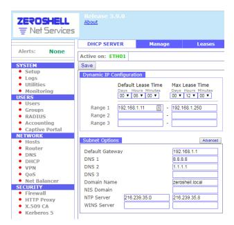
Figure 4.17: Zeroshell's Dynamic Host Configuration Protocol (DHCP) server configuration
