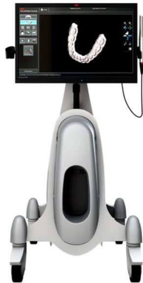
Figura 3.10: Dental clinic 3D scanner 3M True Definition [25]
