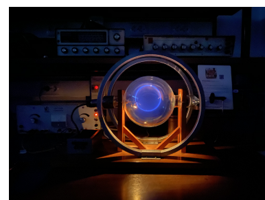
Figure 3.2: Cathode Ray in a dark room. The e-beam with a circle shape.
