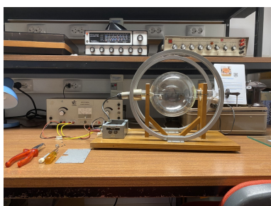
Figure 3.1: Cathode Ray object, with two coils.
