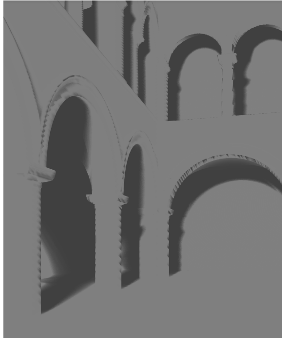
Figure 42: Sponza render using VSM with 7x7 box filter, 7x7 PCSS tap and 1080*2220 map
