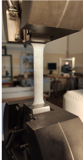
Figure 3.8: Specimen painted with a random pattern, ready for the DIC tensile test
