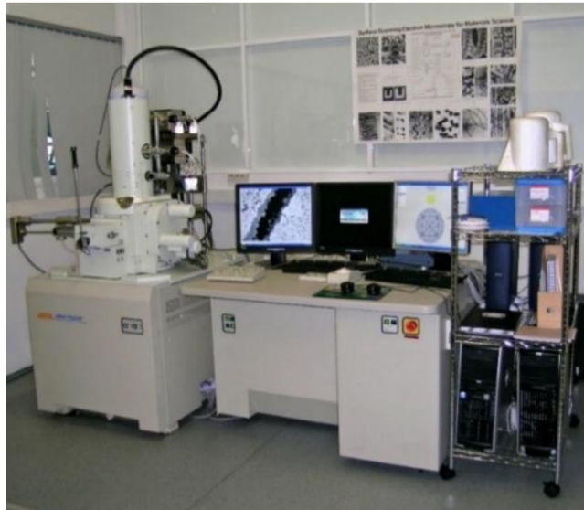
Figure 3.10: Analytical SEM Hitachi S2400, adapted from [40]
