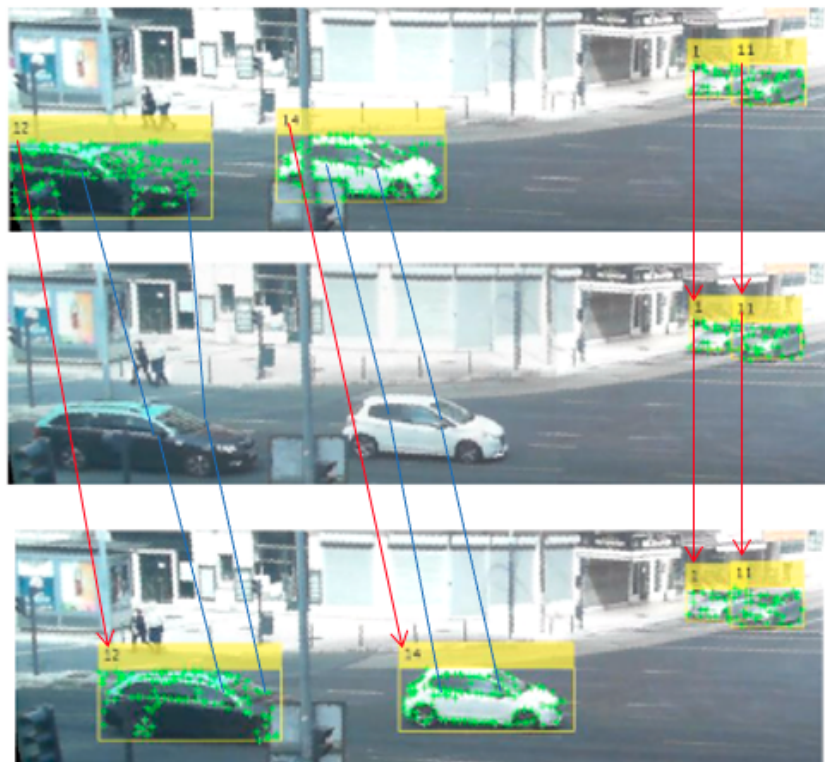
Figure 3.1: Example of the problem and proposed solution. Top image - Object detector and feature selection identify vehicles and image features inside the bounding box. Middle image - object detectors often miss bluntly. However feature trackers can still match corresponding points (blue line). Bottom image- if objects are detected again, the feature tracker allows the association of the correct object (red lines).
