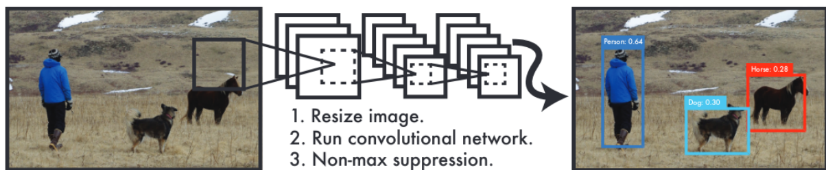
Figure 2.3: The YOLO Detection System. The system (1) resizes the input image to 448 \times 448 , (2) runs a single convolutional network on the image, and (3) thresholds the resulting detections by the model's confidence. Source: [34].
