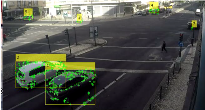
(a) The grey car on the right is identified as 1 and the white car on the left is identified as 2.
