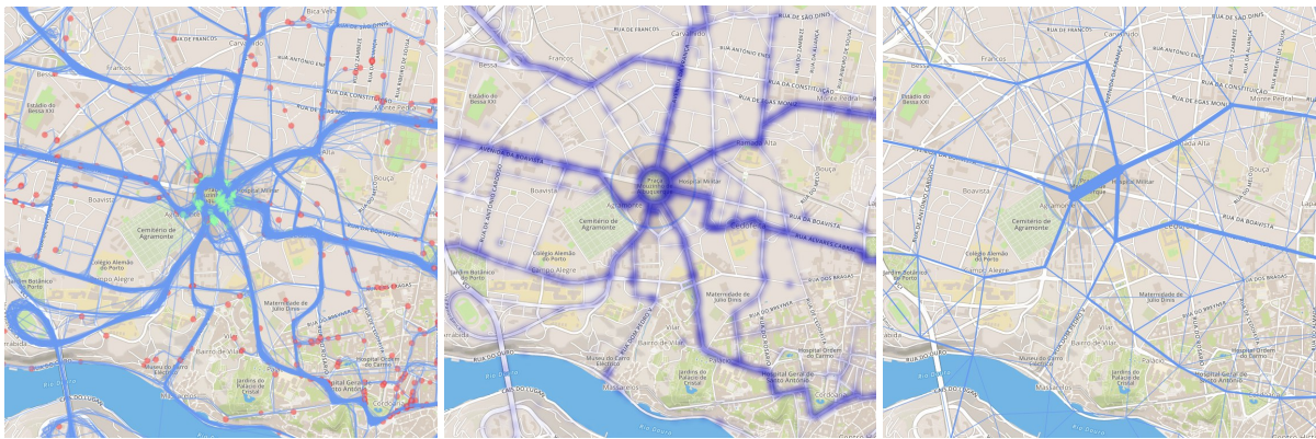
Figure 2.12: Selecting trajectories starting in Praça Mouzinho de Albuquerque, Porto (roundabout in the center). Start points in green and end points in red. From left to right: raw trajectory data, heatmap and welded graph. From TrajAnalytics (Zhao et al., 2016).
